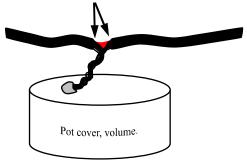
Solution for 'A': For open circuit: Rework the solder points on the baseplate of the pickup, being careful not to melt the Red inner of the attached cable. Wipe the tip of the iron across the solder points in the direction of the small section of the point. Do not apply heat for longer then 3 seconds. If still open circuit it could mean an accidentally broken coil wire caused by taking the cover off without undue care. Remove the cover
